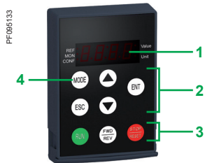
Remote display terminal with cover open
